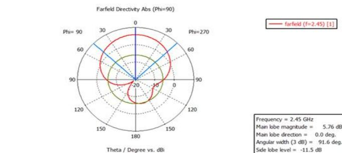
Figure 6. Simulated Radiation pattern at 2.45 GHz (E – plane)
