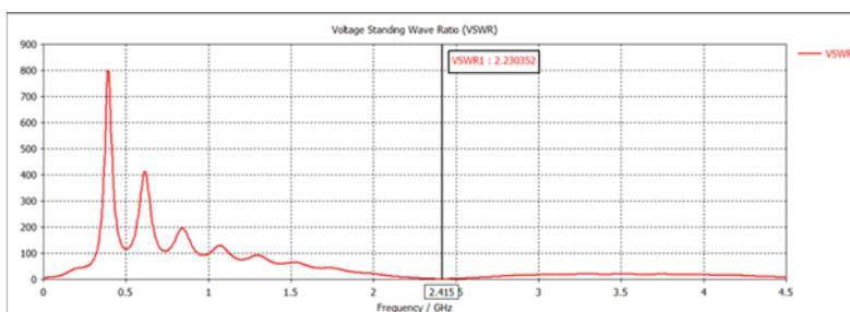
Figure 4. Frequency vs VSWR graphical representation
