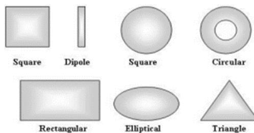
Figure2. Several distinct configurations for microstrip patch antenna [3]
