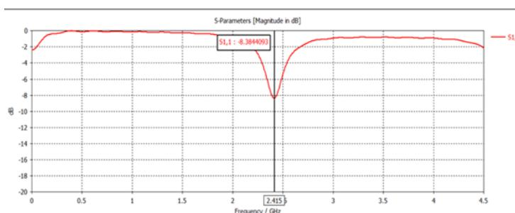
Figure 3. A graph showing return loss versus frequency is presented below
