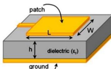
Figure1. Structure of microstrip patch antenna [3]
